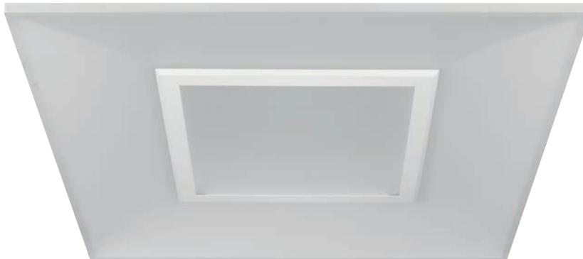
**The DYAD LED is a recessed modular luminaire with symmetric illumination planes. The central diffuser offers glare control through a micro prismatic optic. The outer diffuser is manufactured from a polar white diffuser.**
